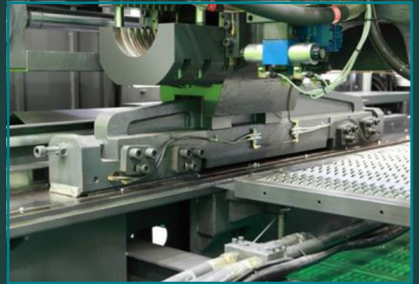
High-rigidity L-shape guide on machine frame, with guiding precision up to 0.05mm, facilitate fast and steady motion of platen.
