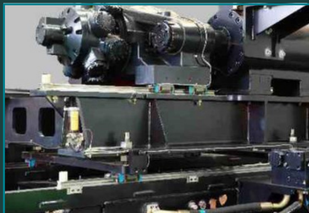
High-rigidity supports and precision linear guides ensure high repeatability
